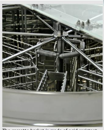
The cassette basket is made of acid resistant stainless steel rods. This design allows the user to secure the frames, stopping the breaking of combs. Cassettes are joined together by springs which allow them to return to the initial position.
